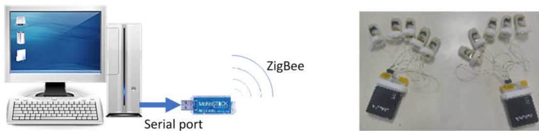
Figure 5: Haptic rendering device communication scheme. Computer broadcasts a command message with ID number. The vibrating part with the correct ID number executes the command for actuation [10][11].
